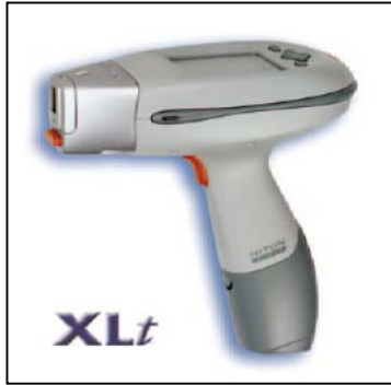
Figure 2. NITON handheld battery-powered XRF analyzer.
